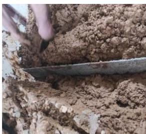
Figure 7: Placing the waterproof wall under the dam model
