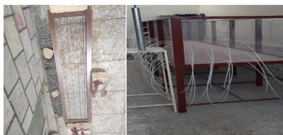
Figure 6: Transparent chamber of the earth dam model and the waterproof wall mold
