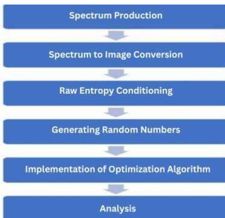
Figure (1): Method of extracting the spectrum of 5G from each 5G Internet of Things device.
