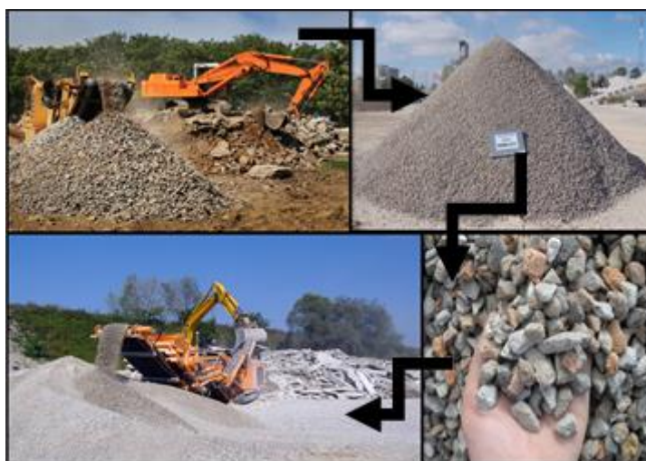
Figure (1) The Production Cycle of Recycled Concrete
